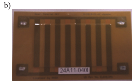
Fig. 6. The IDT designed in the CAD-IDT: (a) layout of electrodes and (b) manufactured prototype
