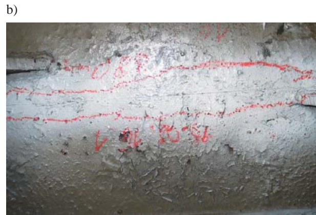
Fig. 3. Cracks of the crane beam revealed by means of the magnetic-powder method: a) type „Z 1 ” joint 120 mm long; b) type „O” plate under the rail, 380 mm long
