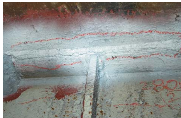
Fig. 4. Fillet weld crack of the crane beam type „B” 240 mm long, detected by the magnetic-powder method
