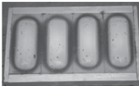
Fig. 5. The macroscopic view of the self-reclamation effect observed for the moulding sand with BioCo2
