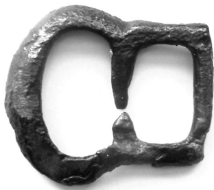
Fig. 7. Bronze buckle, Zesławice (Site 63), 600 AD. a) the view, b) the X-ray spectrum with identification lines for copper, zinc, tin and lead. Concentration of elements: copper – 84%, zinc – 9%; tin – 2%; lead – 4%; other admixtures – 1%
