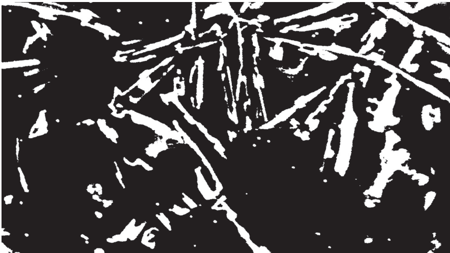
Fig. 6. Binarization of AlSiMg alloy microstructure in initial state using Aphelion software
