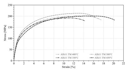
Fig. 6. Stress-strain curves plotted for the feedstock composed of AlSi11 alloy chips extruded at different temperatures
