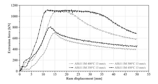
Fig. 2. Force characteristics as a function of ram displacement during extrusion of the AlSi11 IM alloy
