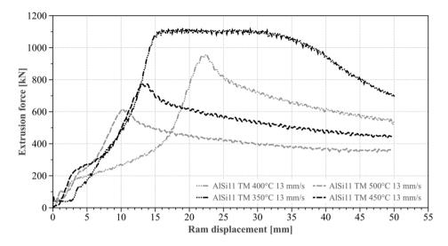
Fig. 3. Force characteristics as a function of ram displacement during extrusion of the AlSi11 TM alloy
