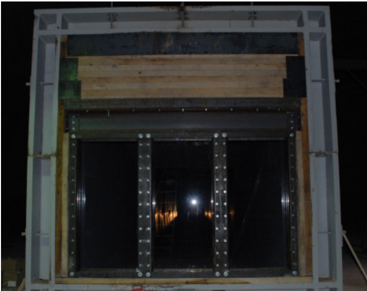
Fig. 2. Completed Half-Width Scale Polycarbonate Wall Installation
