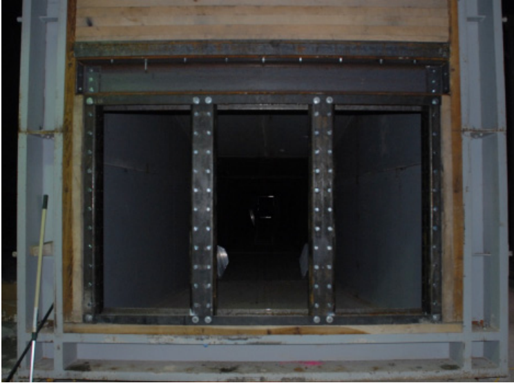
Fig. 1. Half-Width Scale Steel Framing Installed in the Reduced Opening
