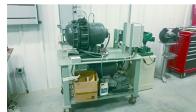
Fig. 4. Explosive chamber used in flame extinguishing experiment.
