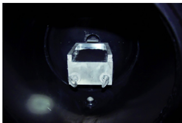
Fig. 8. Sample tray installed in explosive chamber loaded with coal dust.
