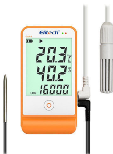
Figure 3.18. Eitech GSP6 data logger
