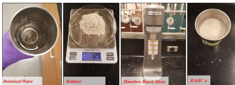
Figure 3.23. Equipment used to prepare and mix the basic A fluid.
