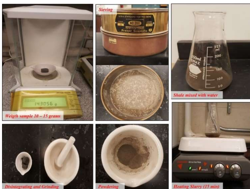
Figure 3.8. CEC shale slurry preparation.
