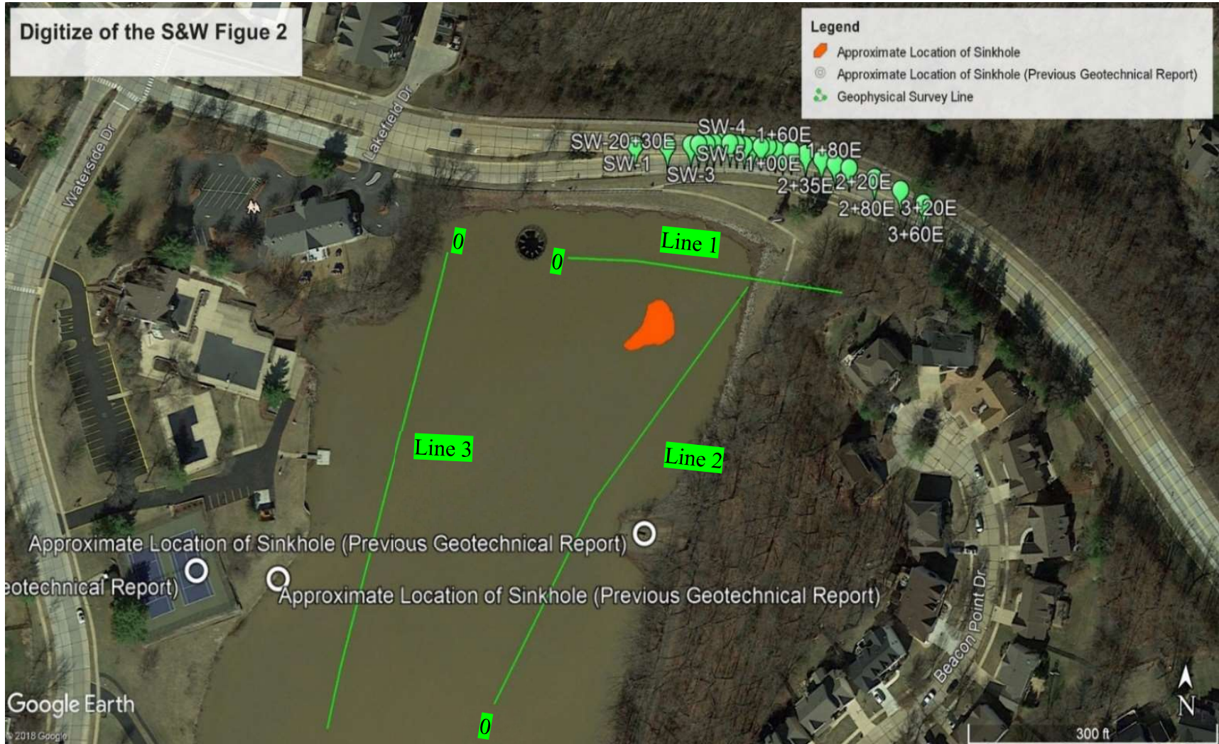
Figure 1.8. Digitize version of the Shannon & Wilson’s surveys. The green line represents ERT traverses; the orange area represents the location of the sinkhole that opened on June 4, 2004.
