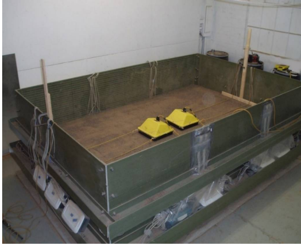
Figure 2.1. The Experimental tank was constructed with no metal and filled with horizontal layers of soil. In this figure, 250 MHz antennas are being moved over dry sand.
