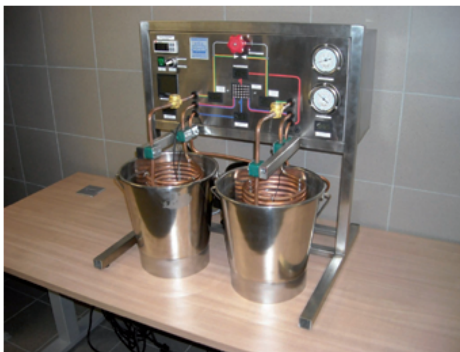
Fig. 4. Didactic heat pump, water-water of the direct evaporation type
