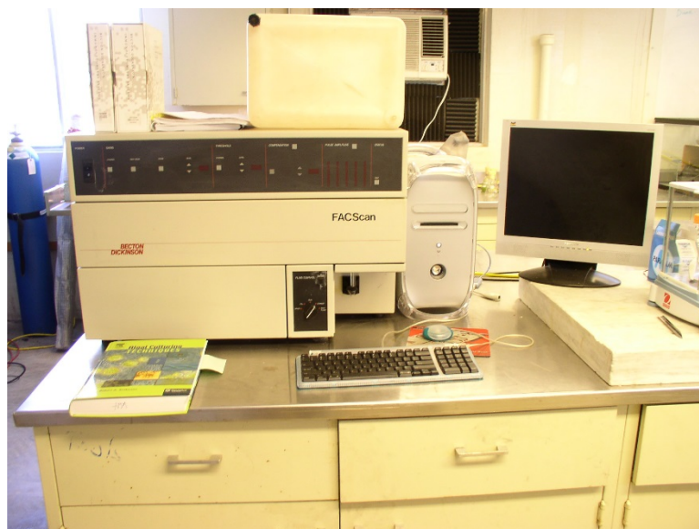
Figure 3.9. FACScan flow cytometer used for enumeration of microalgae cells grown in this study.
