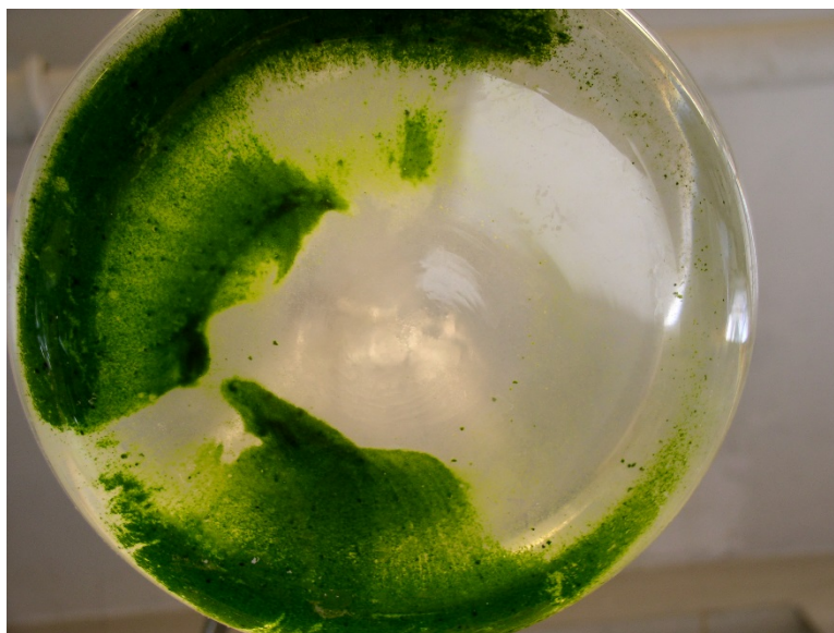
Figure 5.2. Example of biofilm formed with constant illumination under blue (450 nm) light experiment.
