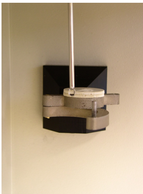
Figure 3.14. Picture of a drop of sheath fluid forming at the end of the SIP tube.
