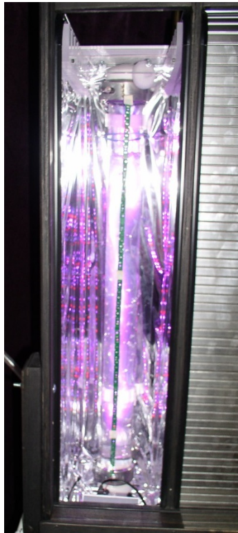
Figure 3.29. Prototype of glass photobioreactors that replaced original extruded acrylic type. Note endcaps are constructed out of PVC and not PEI plastic in this model.
