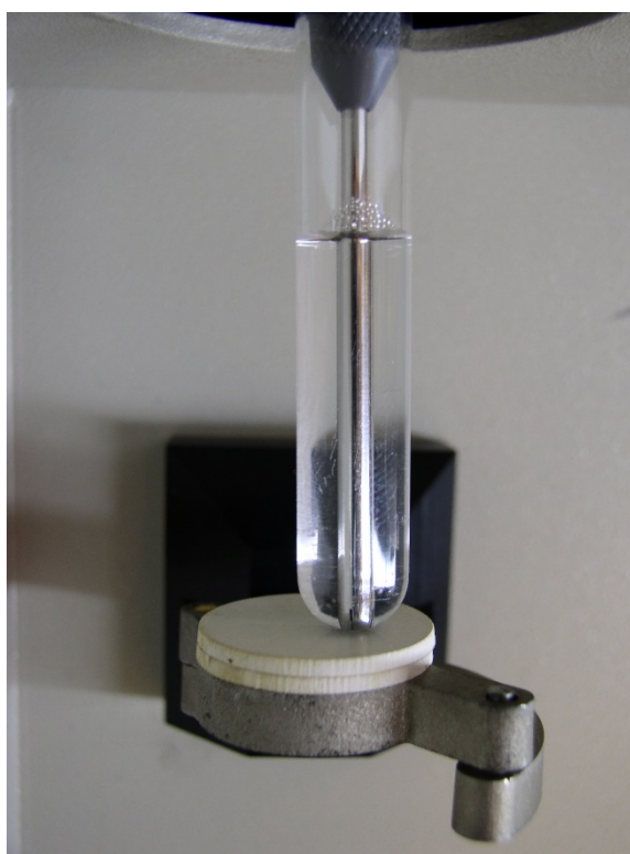
Figure 3.12. Modified SIP arm installed on the FACScan in standard configuration.
