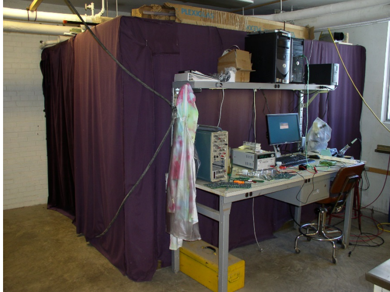
Figure 3.19. Finished darkroom with black-out curtain applied.
