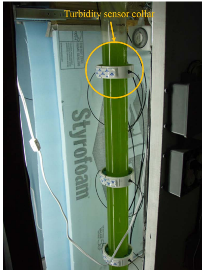
Figure 3.7. Initial, rudimentary turbidity sensor previously built for the project.
