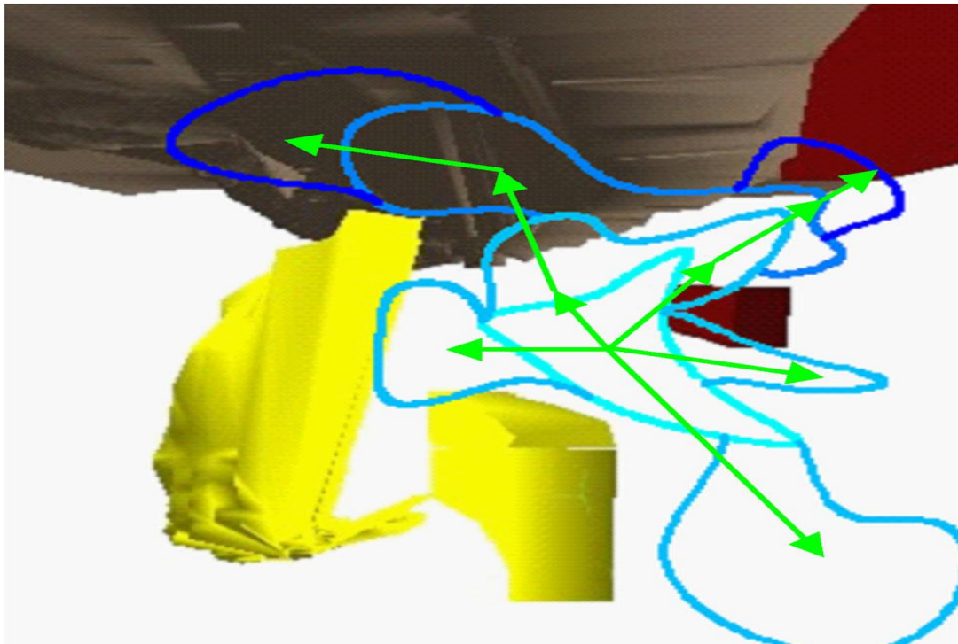
Figure 2.11 Direction and range of the fault activation (—Up to December 5, 2009, —Up to January 1, 2010, —Up to February 12, 2010, —Up to March 23, 2010) [12]
