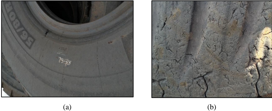
Figure 1.4. Fatigue failure Forms Initiated by Rock Cuts in (a) Sidewall, and (b) Tread
