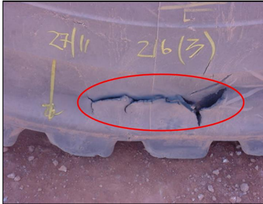
Figure 1.3. Mechanical Separation in a 55/80R63 Tire [10]
