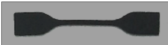
Figure 5.3. A Typical Simple Tension Specimen Geometry
