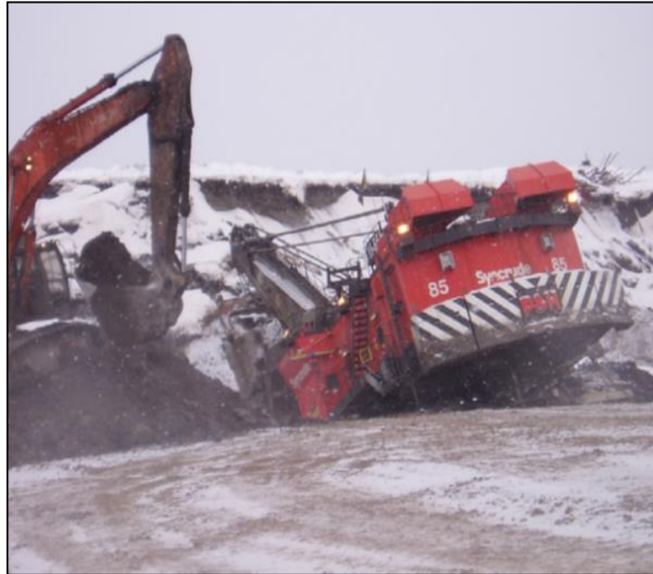
Figure 1.5. Sunk Electric Rope Shovel on Firm (Frozen) Near-Surface Oil Sand Ground [19]
