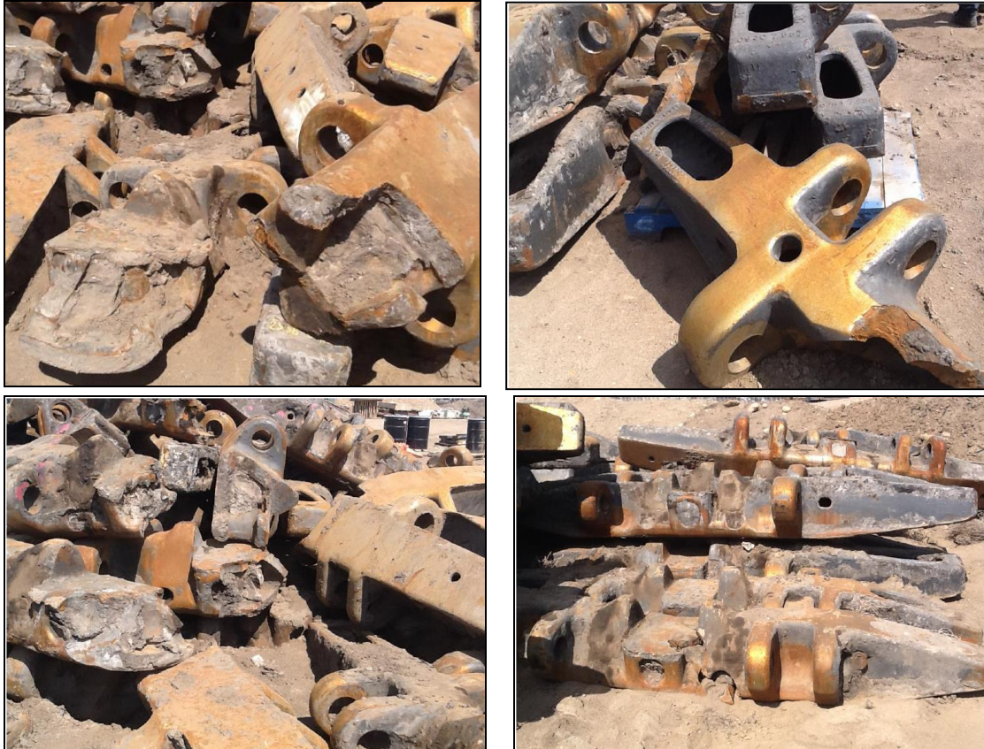
Figure 1.6. Wear and Fracture in Crawler Shoes (Syncrude, 2014)
