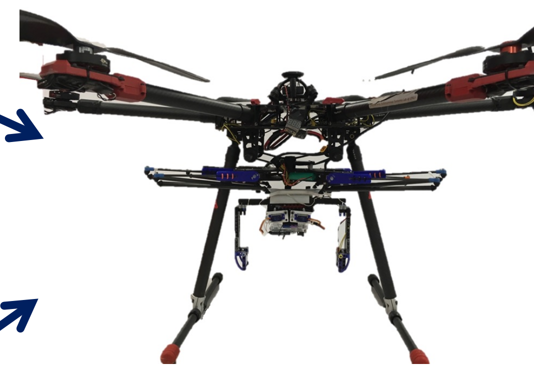
(C) Mobile Manipulating UAV Concept with Parallel Manipulator-Gripper
