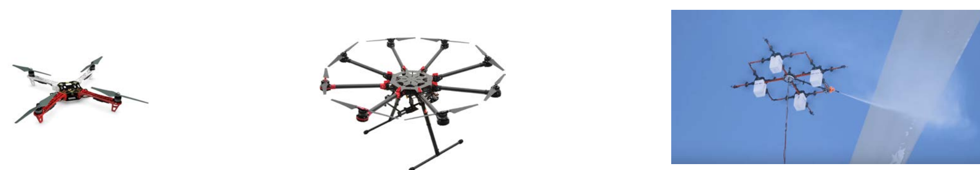
Fig. 1. Hose mounting is modeled with some: horizontal and vertical offset from CoG, angle from UAV's roll and pitch origin, and force magnitude as function of tank PSI.
