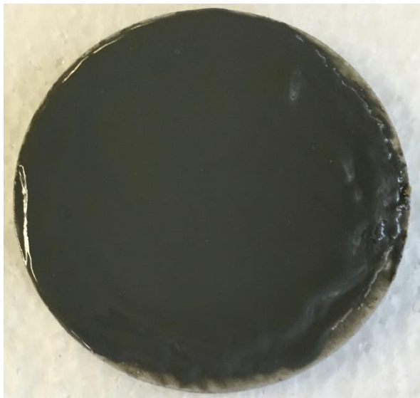
Figure 4-4. A shale sample was exposed to the fluid of test #2 (2% Bentonite + 4% Fly Ash)
