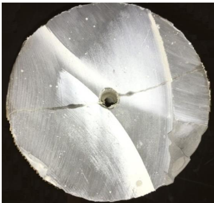
Figure 3-1. Symmetric and bi-wing fracture created around the wellbore for Test #7
