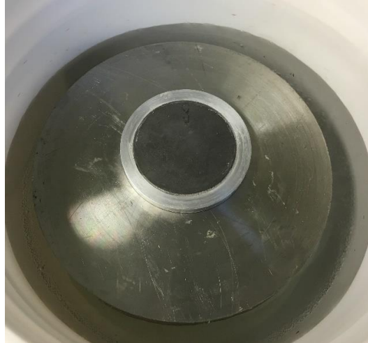
Figure 3-2. A shale sample were secured with epoxy in a casing and were placed in humid chamber couple of hours before PTT experiment
