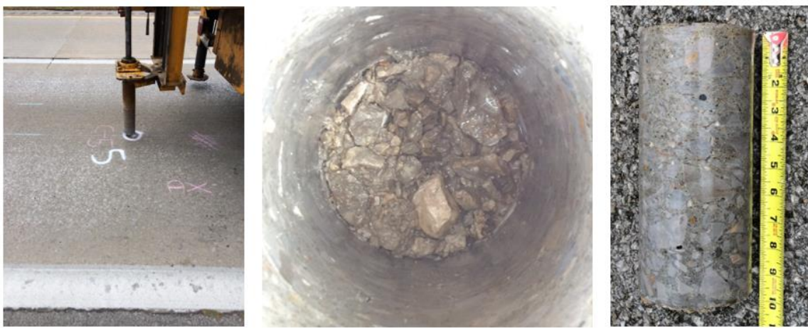
Fig. 5. Photos of core #5 retrieved from the experimental segment.
