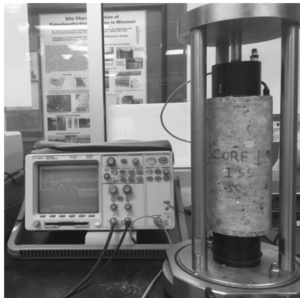
Figure 2. Ultrasonic velocity testing system.
