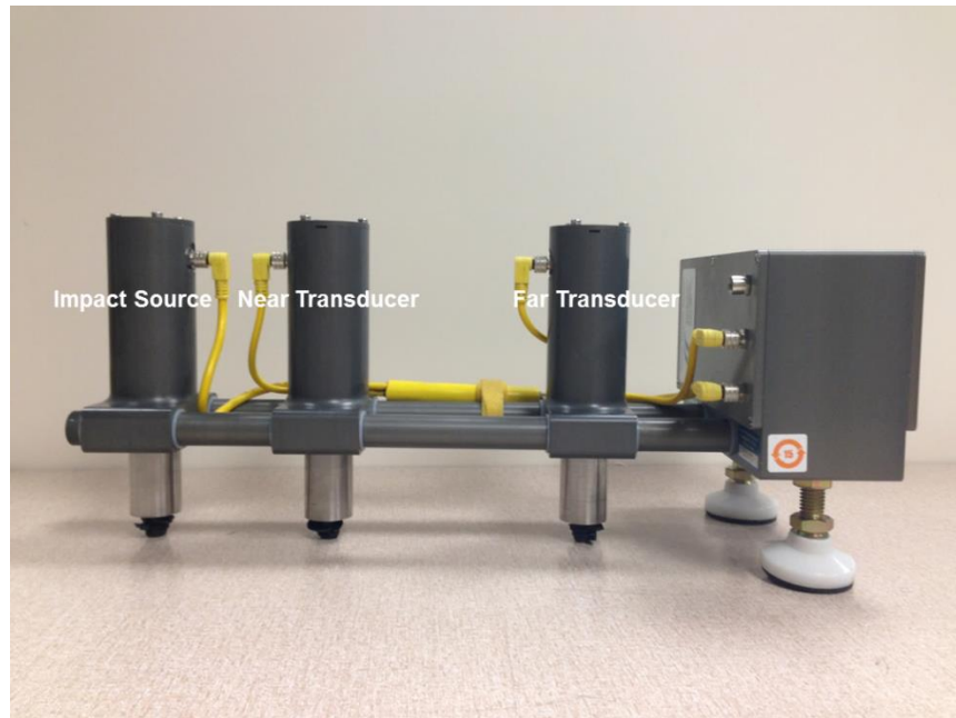
Fig. 2. Portable seismic property analyzer (PSPA).
