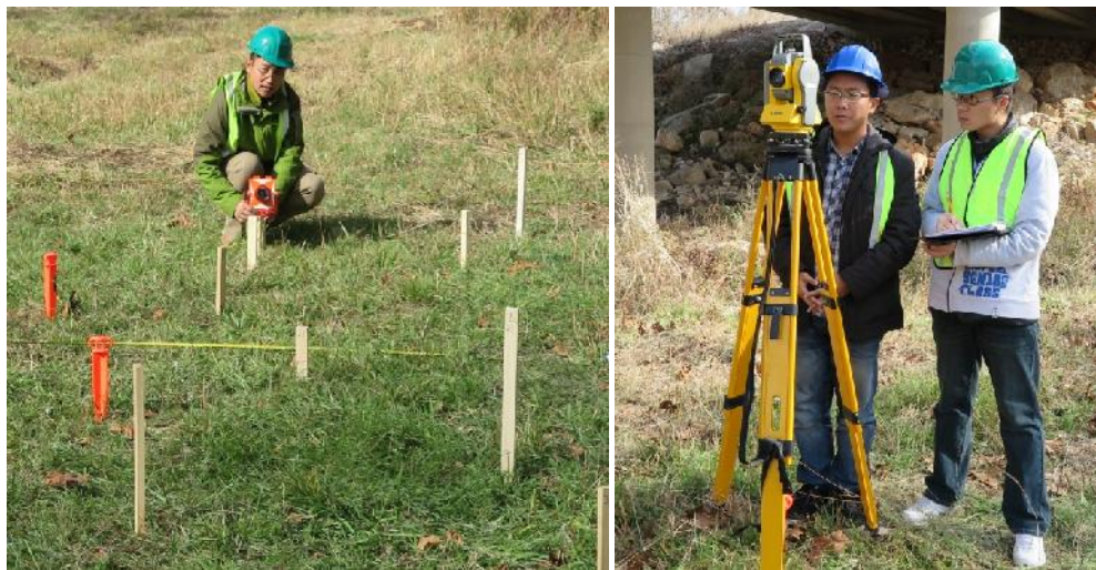
Figure 4.7. Total station and prism for positioning.
