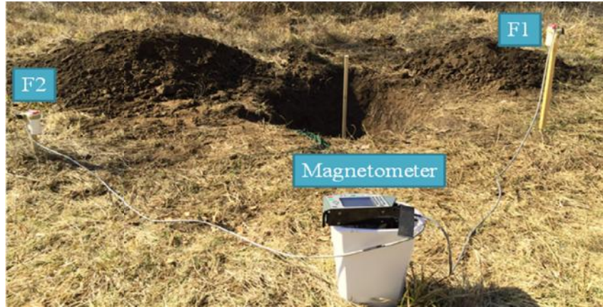
Figure 2.10. Overall arrangement of resetting tests.
