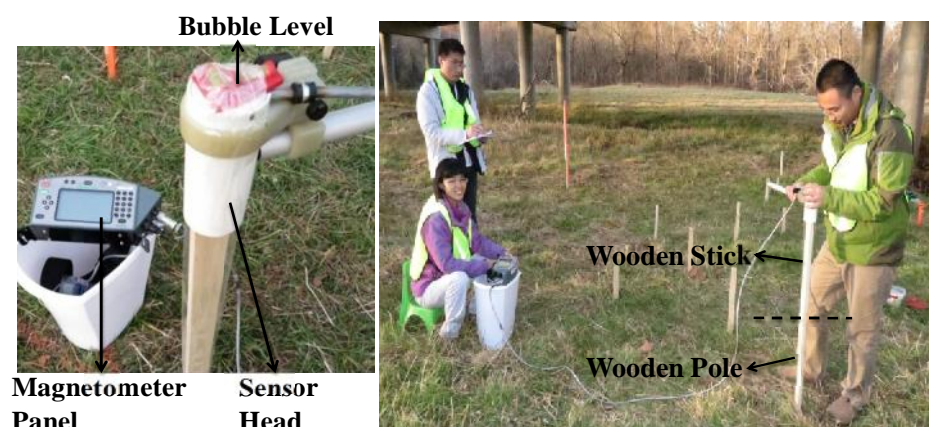
Figure 4.9. Magnetometer setup and operation.
