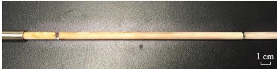
Figure 10. Picture of the semi-rigid CCFPI temperature sensor.
