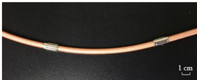
Figure 4. Picture of the flexible CCFPI temperature sensor.
