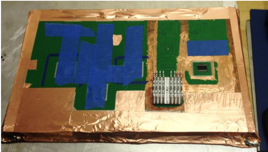
Figure 5.3. Clock buffer IC board for validation
