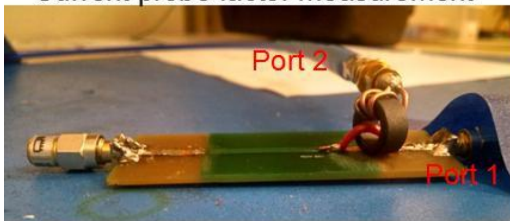
Figure 3.3. Current probe characterization
