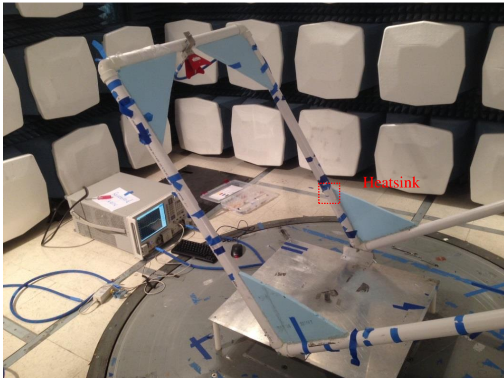
Figure 4.1. Maximum far field measurement setup
