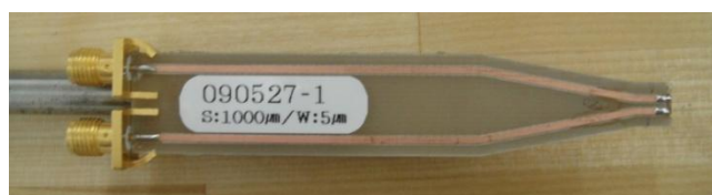
Figure 2.1. Overall view of GMI probe
