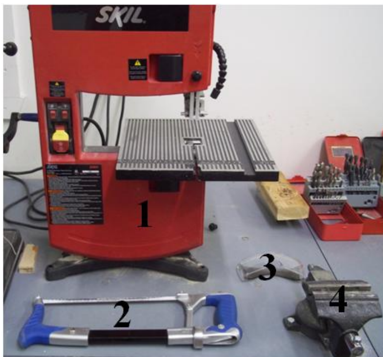
Figure D.2. Setup for cutting sample using band saw. SKIL 9-inch (229 mm) Benchtop 2 Speed Band Saw is indicated as 1. Hand saw is indicated as 2. Safety goggles are indicated as 3. Vice grips are indicated as 4
