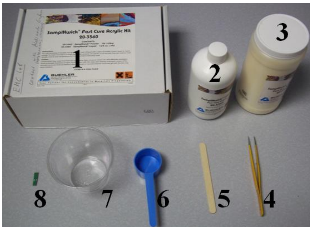
Figure D.7 SamplKwick Fast Cure Acrylic Kit 20-3560 with indicated parts
