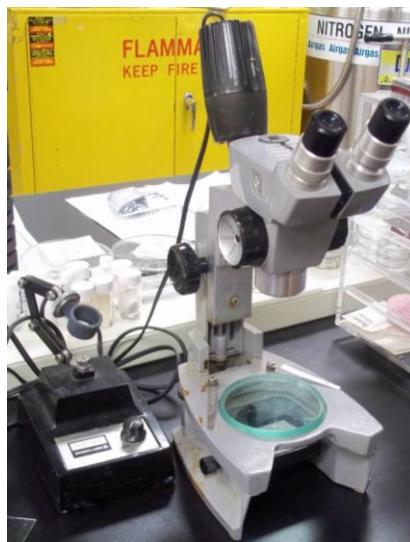
Figure D.20 Optical microscope with medium magnification
