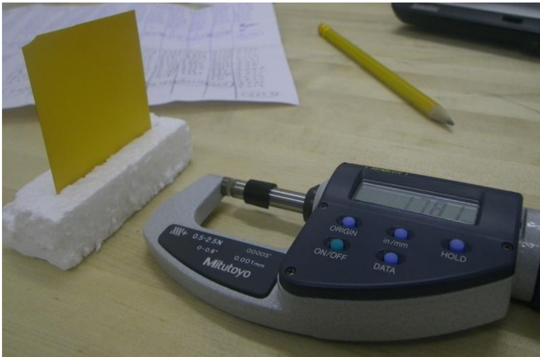
Figure G.2 Sample thickness measurement
