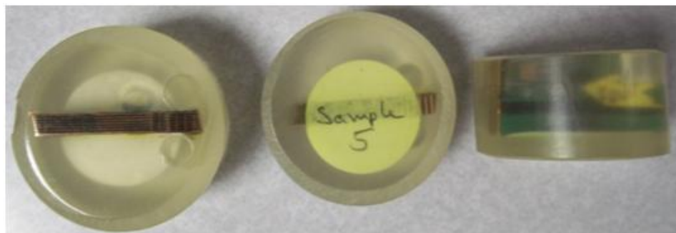
Figure D.10. Example of labeling the sample, and using plastic holders
