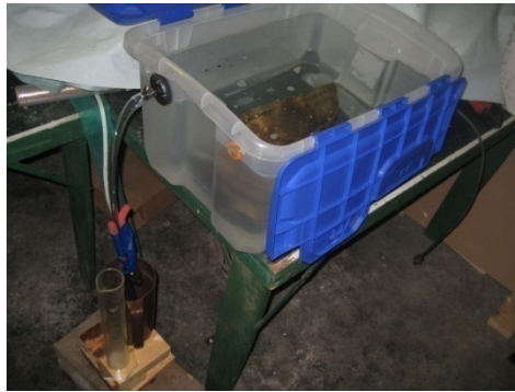
Figure 3.16. Water Immersion Volume Test.
