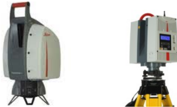
Figure 2.5. Image of LiDAR Scanners Used in Project. ScanStation2 (Left) and HDS6000 (Right) (Leica Geosystems).
