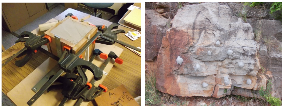
Figure 3.18. Clay Rockfall Simulation Test Setup. Small Box Used for Measuring the Clay (Left) and The Rock Outcrop With Clay (Right).
