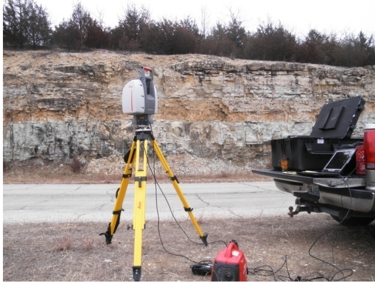
Figure 3.3. Site 1 Setup (ScanStation2 placed securely on tripod, powered by EU1000i Honda generator, and operated using Cyclone software on laptop).
