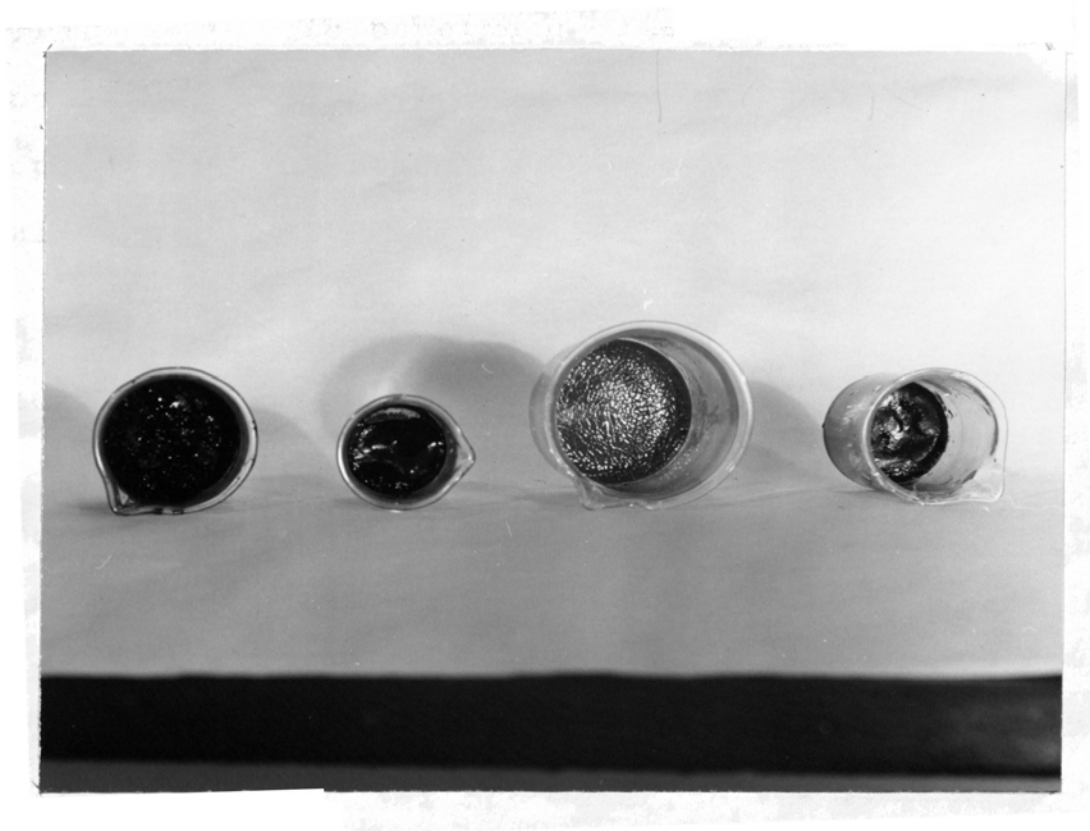
Plate VII. Air Dried Gel Showing the Fracture Pattern.
