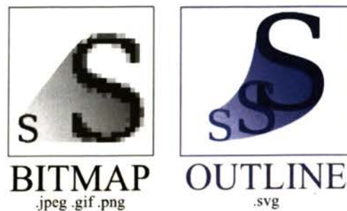
Figure 1.3. The difference in clarity between bitmap and scalable vector images at variable scales (Cheng, 2006).
