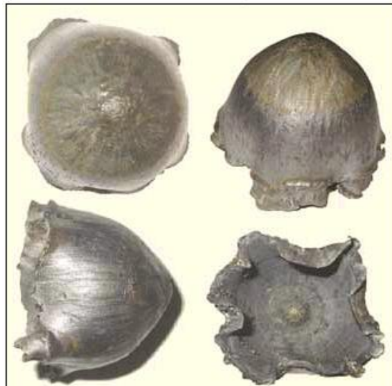
Figure 2.6 Figure collected during Explosively Formed Projectiles (Dr. James N. Willson; Dr. David E. Lambert, and Mr. Joel B. Stewart, 2006)
