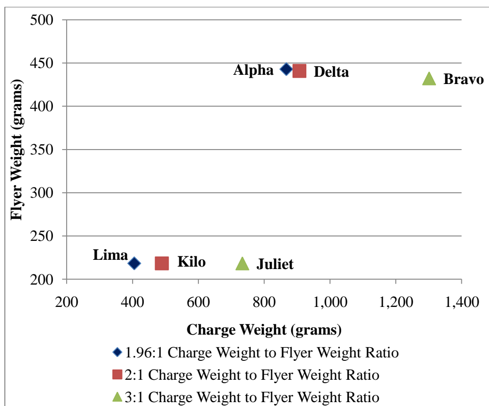
Figure 3.8 Charge Weight to Flyer Weight Ratios
