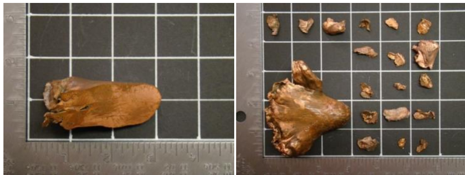
Figure 5.4 Projectiles Produced From the Alpha EFP Design
