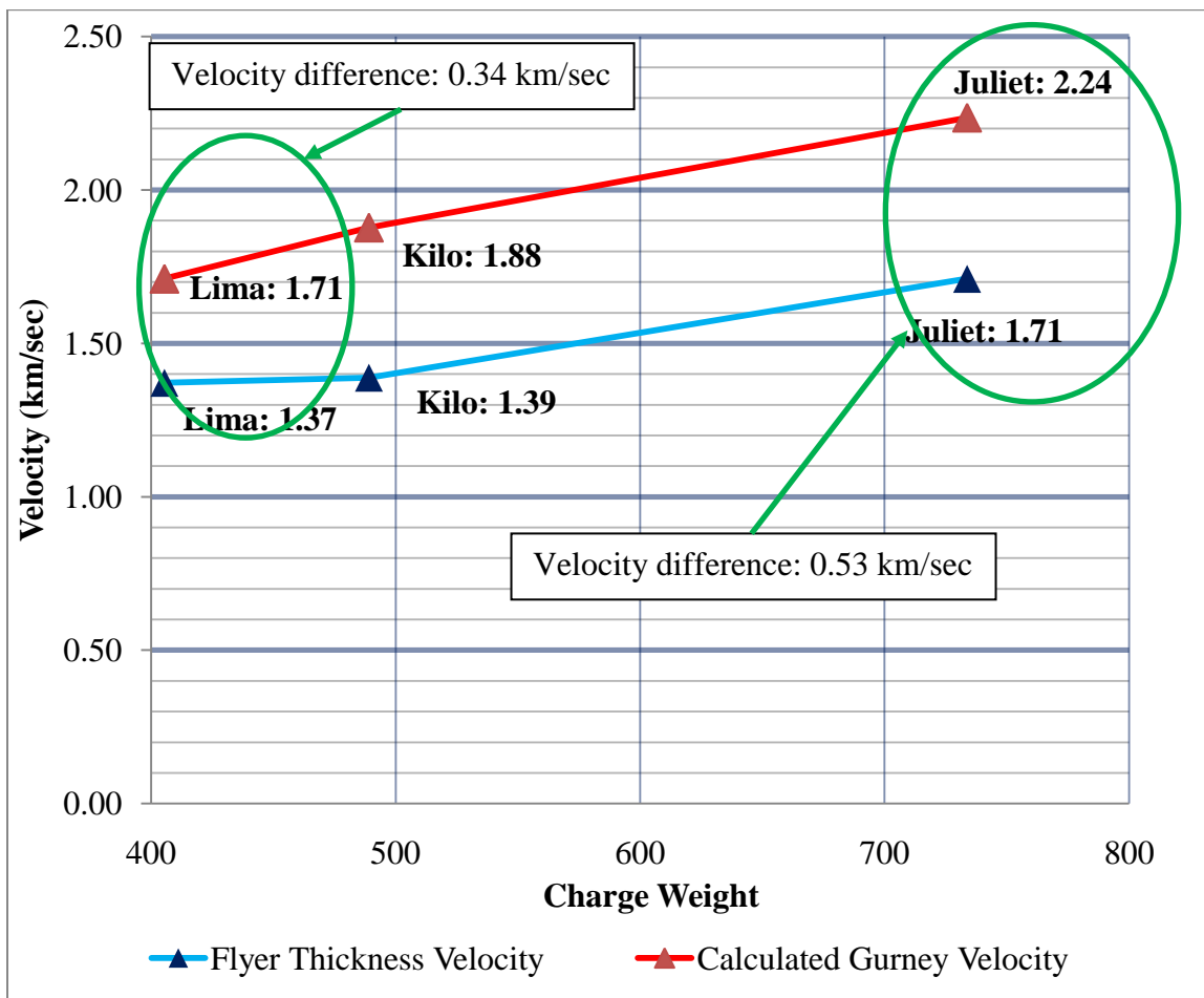
Figure 5.15 Flyer Thickness Velocity Data
