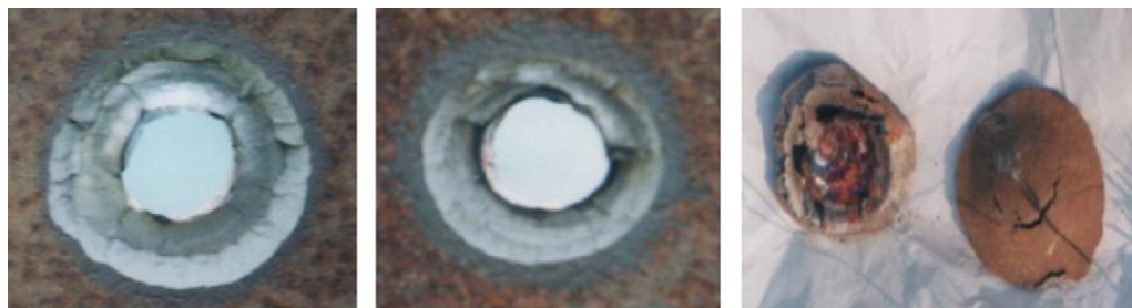
Figure 2.4 Penetration of a 2.54 cm Steel Plate (Wu, 2007)
