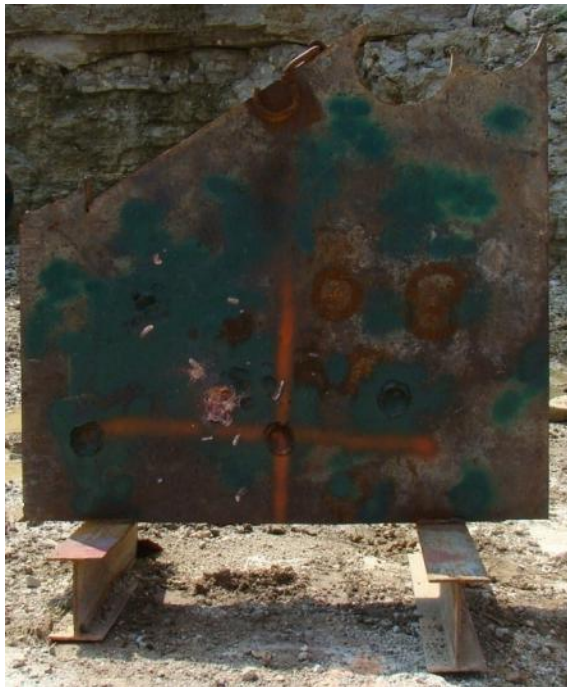
Figure 4.3 Target for Penetration Test
