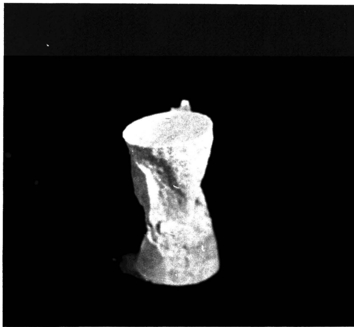
Figure 10. Photograph Showing The Fracture Pattern in a Sandstone Specimen
