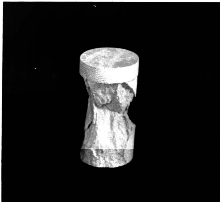
Figure 17. Photograph Showing the Fracture Pattern in a Two-Layered ( h_1/h_2=3.0 ) Specimen of Limestone/Dolomite
