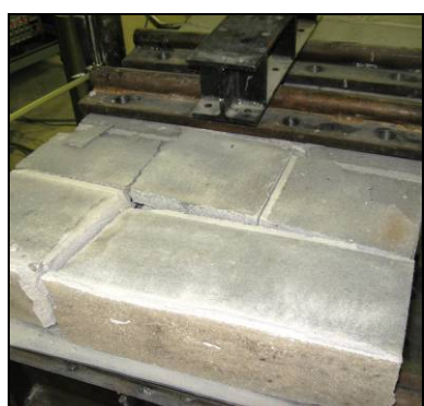
(c) Separation of Masonry
