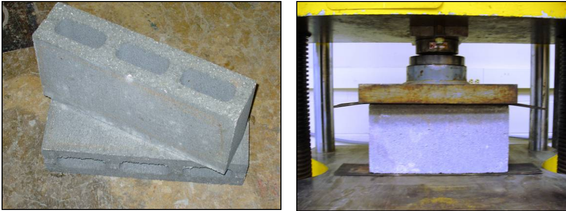
Figure 3.8. Testing of Individual Concrete Masonry Units
