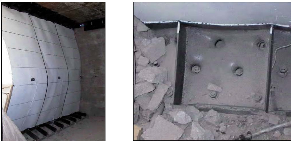
Figure 2.3. Steel Plate Catcher System (Bogosian and Crawford, 2000)
