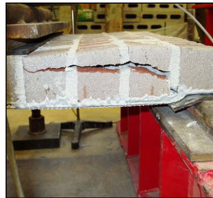
(b) Flexural-Shear Cracking
