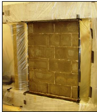
(a) Primed URM Wall
