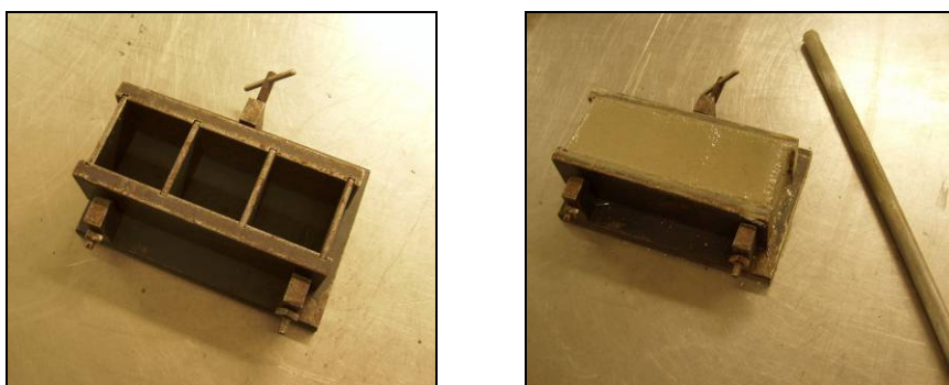
Figure 3.5. Mortar Cube Casting
