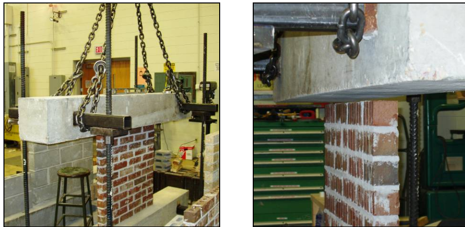
Figure 5.3. Placement of Upper Boundary Element
