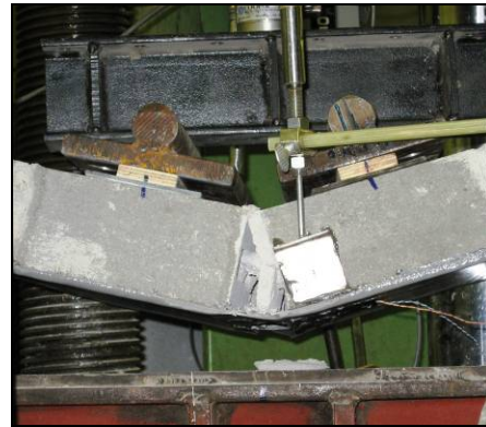
(b) Growth of Crack Width
