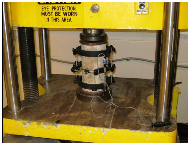
Figure 3.11. WF-FA Compression Testing
