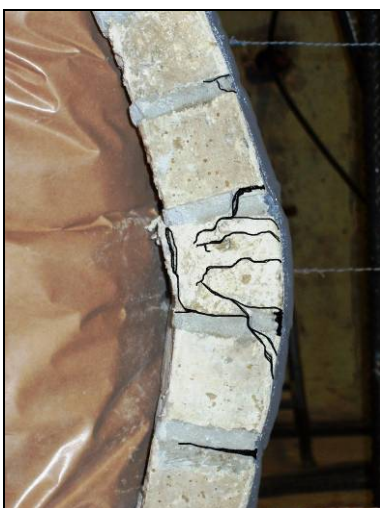
(b) Flexural Cracks in WF-FA
