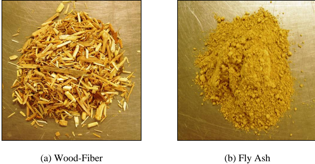
Figure 3.9. WF-FA Primary Materials
