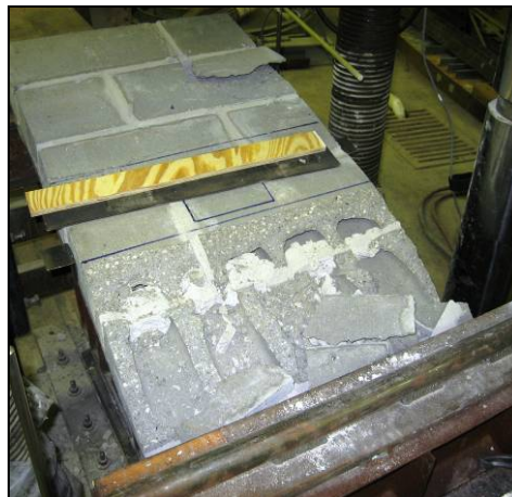
(c) Fracturing of Masonry
