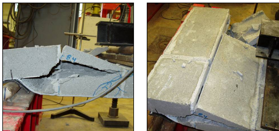
(a) Separation from Polyurea
