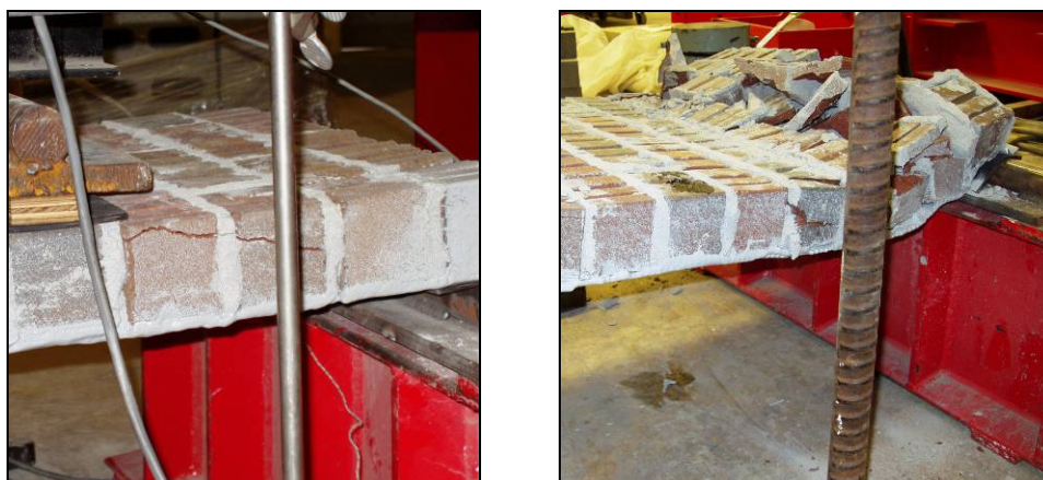
(a) Flexural-Shear Cracking
