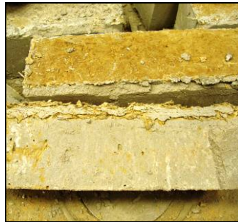
(c) Crushing of WF-FA Brick Units
