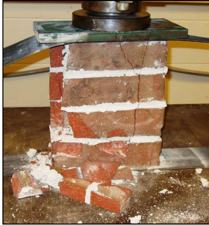
Figure 3.12. Compression Testing of Clay Prism
