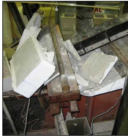
(b) Debonding of Masonry
