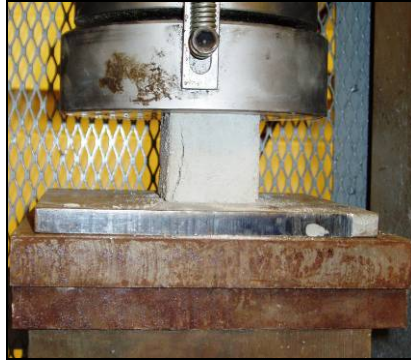
Figure 3.6. Mortar Cube Testing
