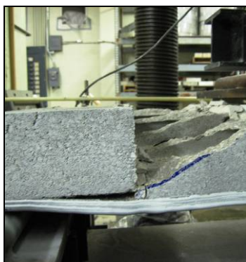
(c) Flexural-Shear Failure
