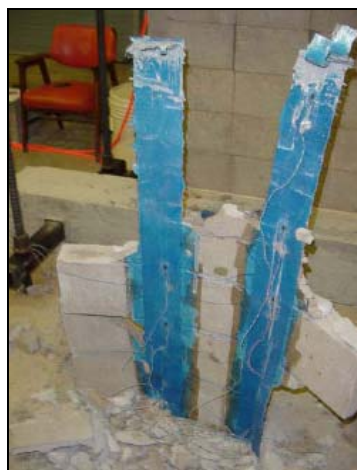
(a) Surface Laminate Retrofit
