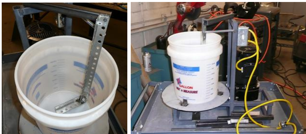
Figure 2.1 Mixing plate and scraper bar shown with an empty mixing bucket
