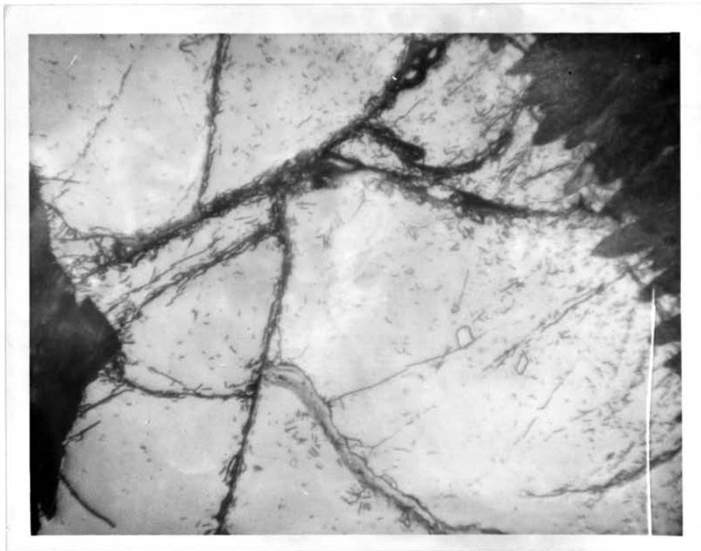
Figure 35. Photomicrograph of a glass-ceramic specimen heat-treated according to point 1.1 (Figure 14) viewed with reflected light under uncrossed nicols. 148X
