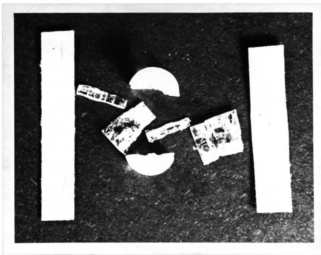
Figure 15. Nonheat-treated \text{SiO}_2\text{-Al}_2\text{O}_3\text{-MgO-Li}_2\text{O} glass cylinder after breaking by the diametral loading technique, shown with loading strips.
