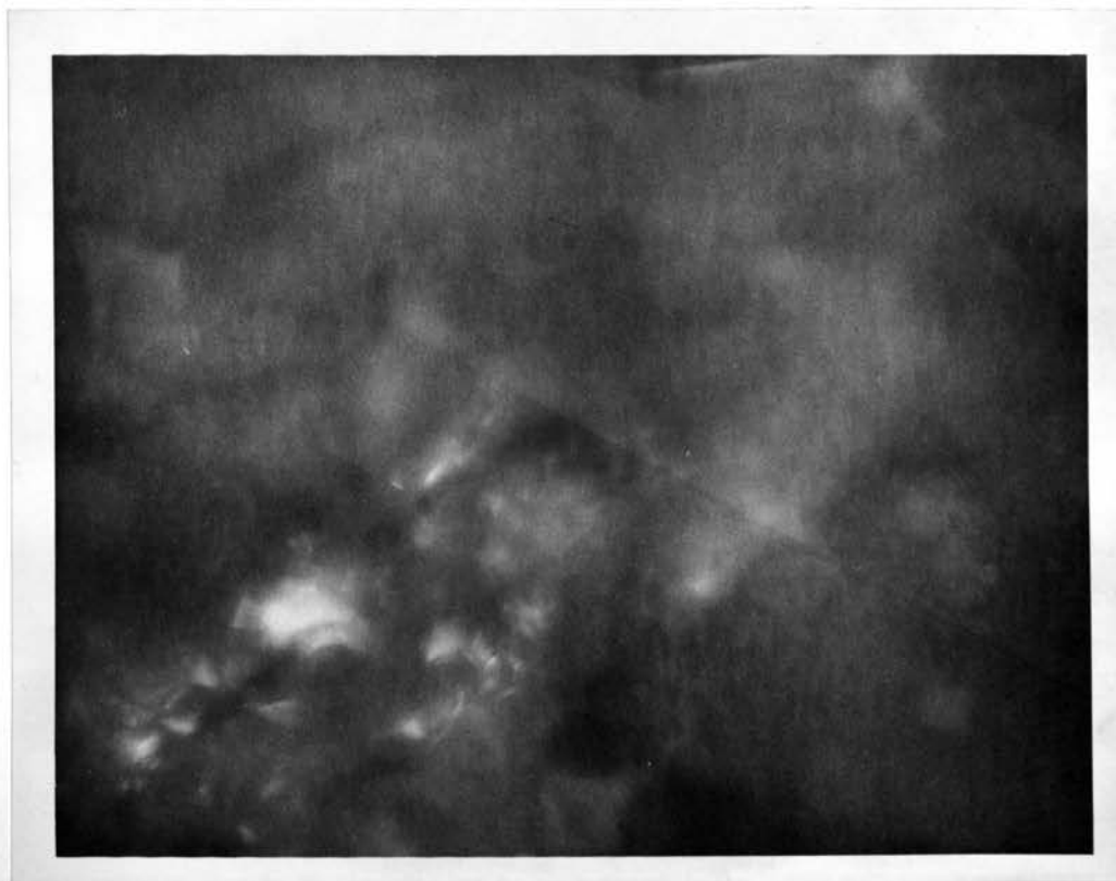
Figure 34. Photomicrograph of a glass-ceramic specimen heat-treated according to point 1.05 (Figure 14) viewed with reflected light under crossed nicols. 170X
