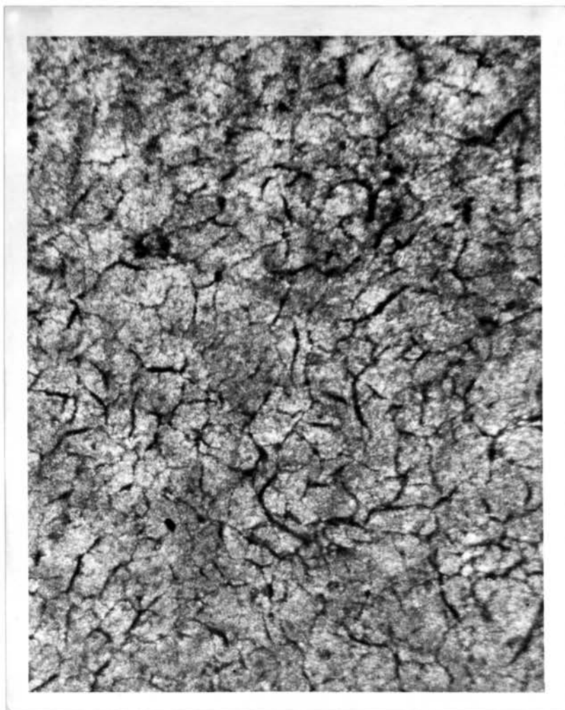
Figure 31. Photomicrograph of a glass-ceramic specimen heat-treated according to point 2.3 (Figure 14), viewed with transmitted light under uncrossed nicols. 27X
