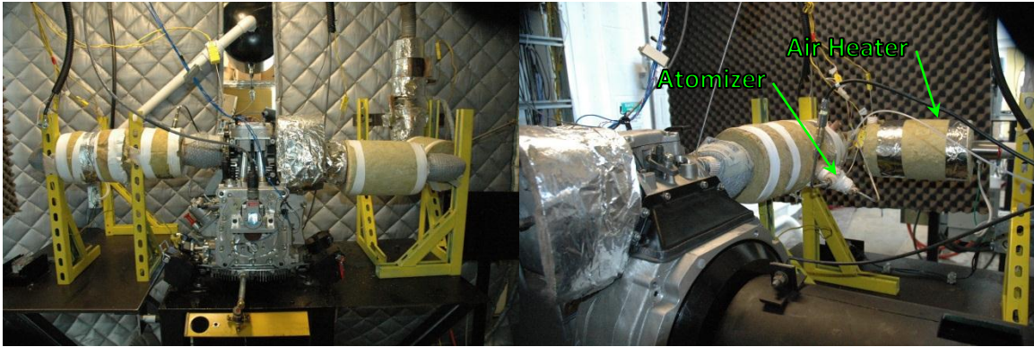
Figure 3.2. Hatz 1D50Z engine setup with the HCCI intake system
