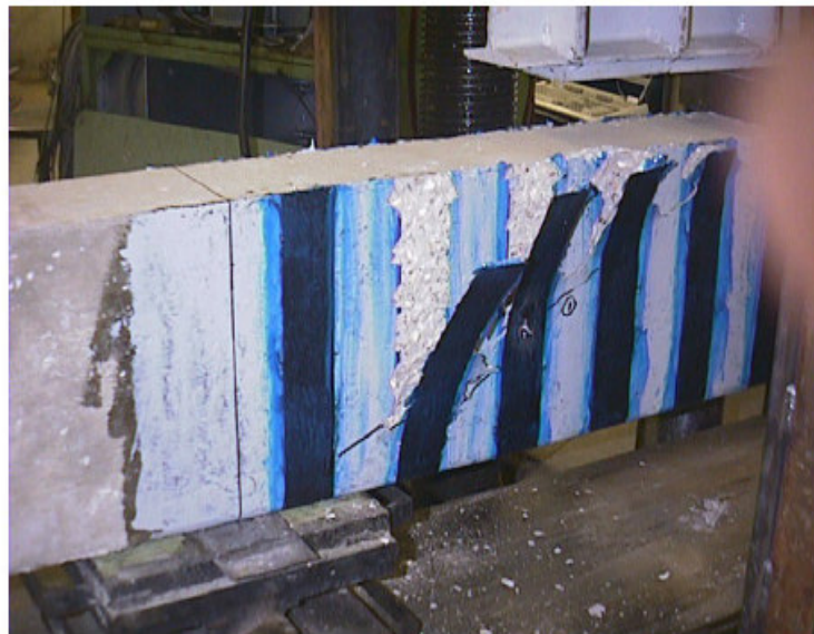
Figure 2.5. Shear Failure due to FRP Debonding (Khalifa, 1999)
