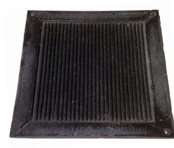
Figure 4.10. Compression molded hybrid composite bipolar plate
