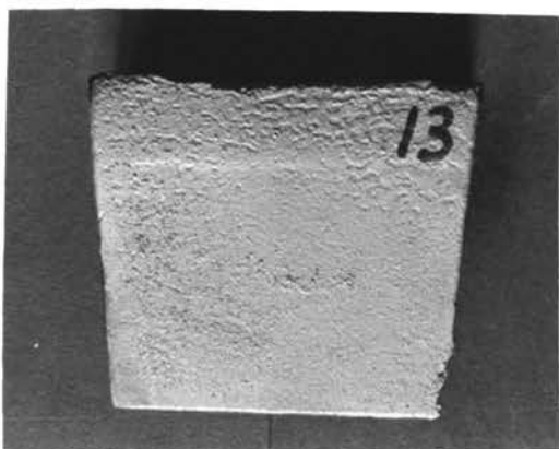
C. Casting #13 30% Magnetite (+325)
