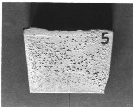
D. Casting #5 50% Magnetite (+65)
