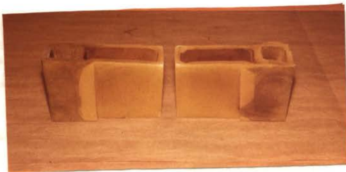
C. Composite molds made with aluminum pattern.
