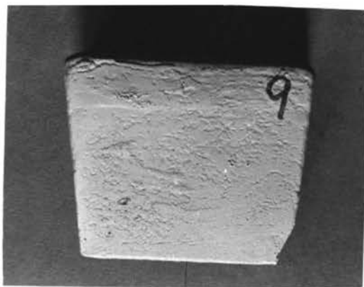
A. Casting #9 10% Magnetite (-325)
