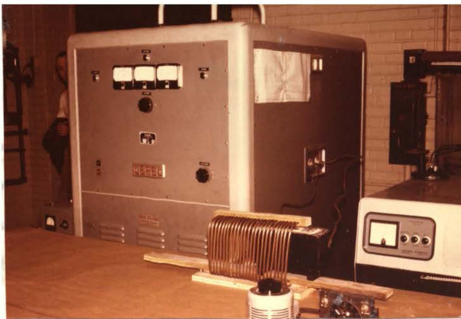
Figure 8. Photographs of experimental apparatus. Note mold being cured in coil.
