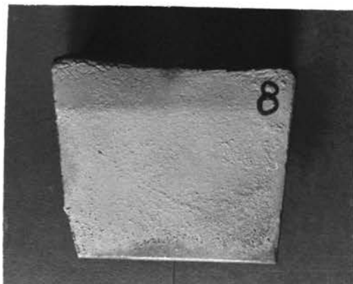
A. Casting #8 10% Magnetite (+65)
