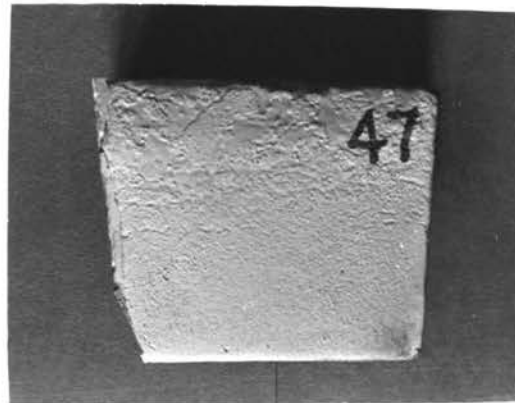
C. Casting #47 20% Magnetite (+100)
