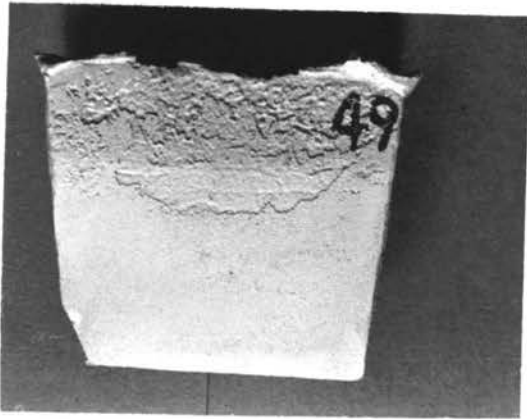
A. Casting #49 Zircon Sand
