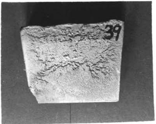
D. Casting #39 Silica Sand
