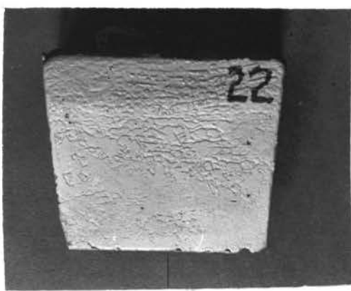
D. Casting #22 30% Magnetite (+325)
