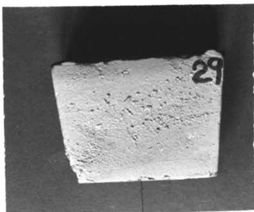
E. Casting #29 50% Magnetite (+150)
