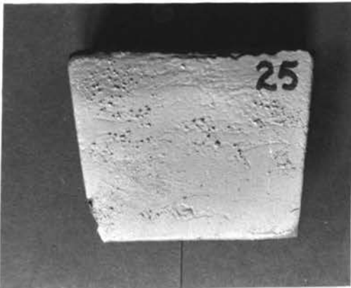
I. Casting #25 50% Magnetite (+200)
