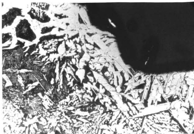
C. Transition area from carburized (left) to uncarburized (right) surface.
