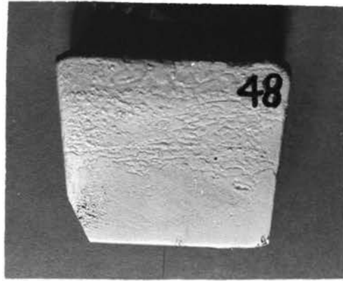
H. Casting #48 40% Magnetite (+200)
