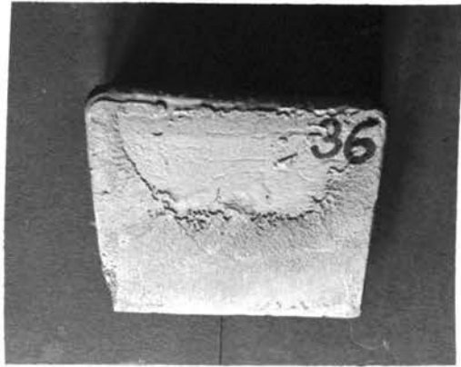
B. Casting #36 Silica Sand
