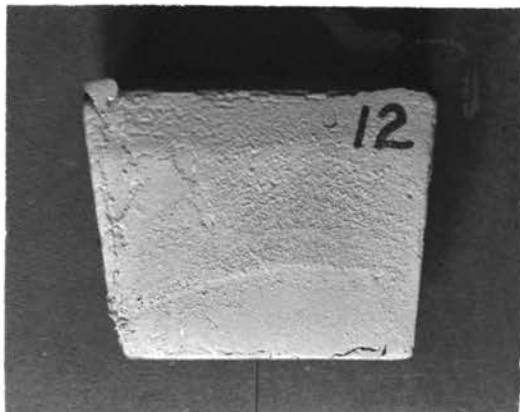
A. Casting #12 10% Magnetite (+150)
