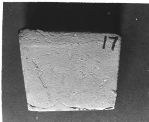
F. Casting #17 30% Magnetite (+200)
