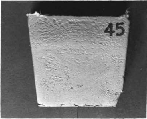
G. Casting #45 40% Magnetite (+200)
