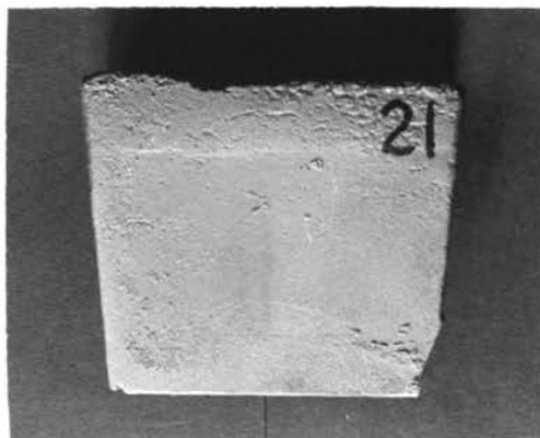
D. Casting #21 30% Magnetite (+150)
