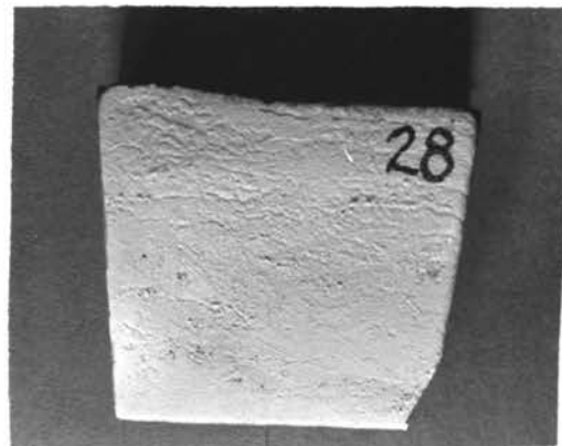
J. Casting #28 50% Magnetite (+200)
