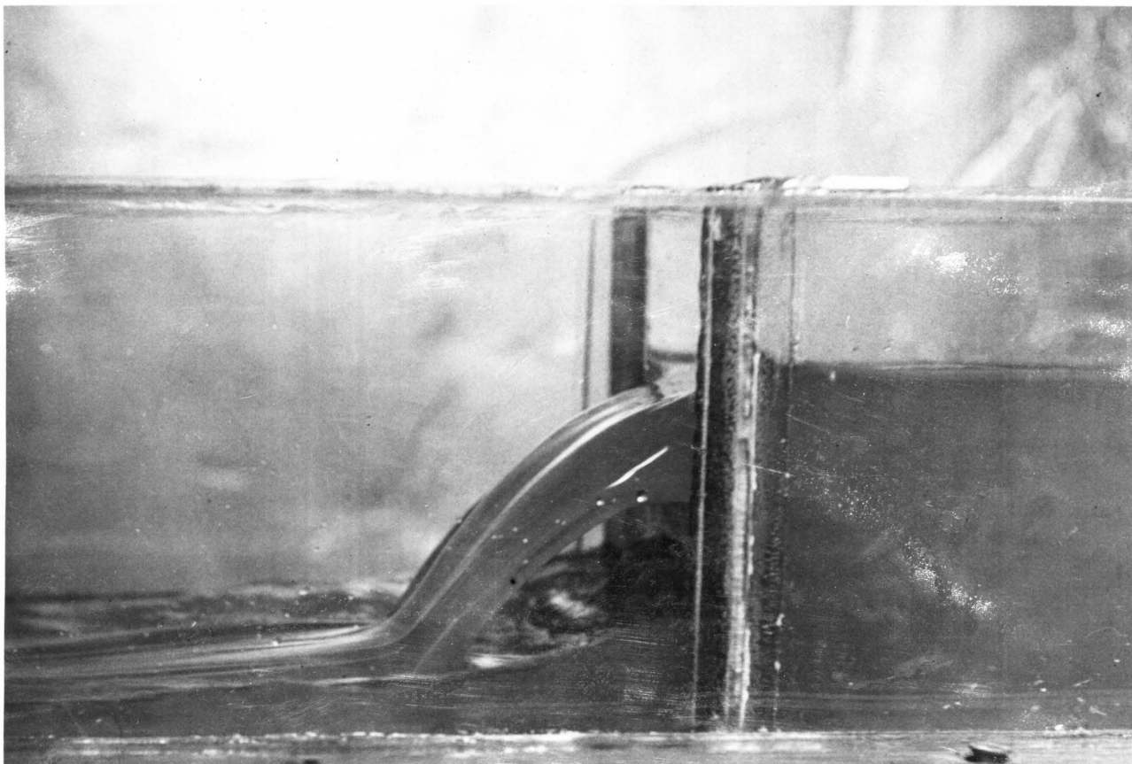
SIDE VIEW OF WEIR NUMBER 2 DISCHARGING.
