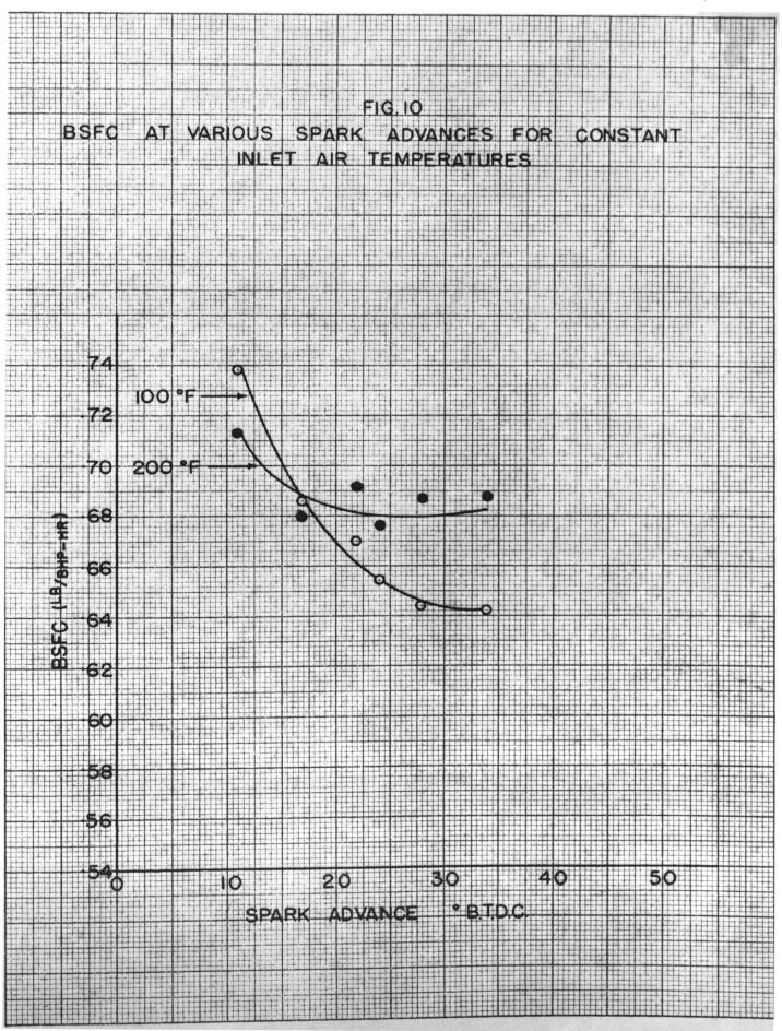
PART V CONCLUSIONS The results of the tests on the engine used for this thesis show that heating the inlet air increase the brake specific fuel consumption at part throttle and at the most efficient spark advances. Besides being more efficient at the cooler temperatures of inlet air the warmer air limits the amount the spark can be advanced due to detonation which also increases the brake specific fuel consumption.
