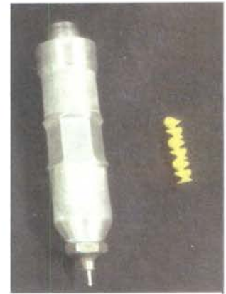
Figure 2: Static mixer (left) with mixing elements (right).
