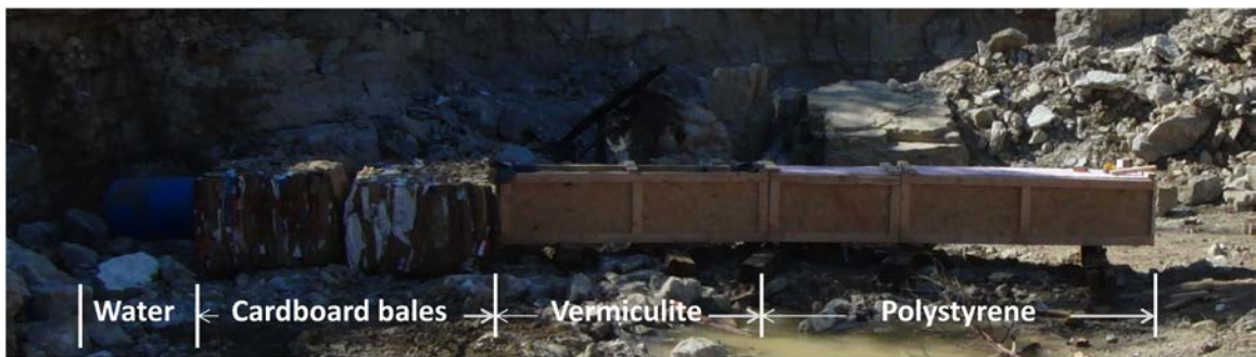
Figure 3.5: Soft recovery system.
