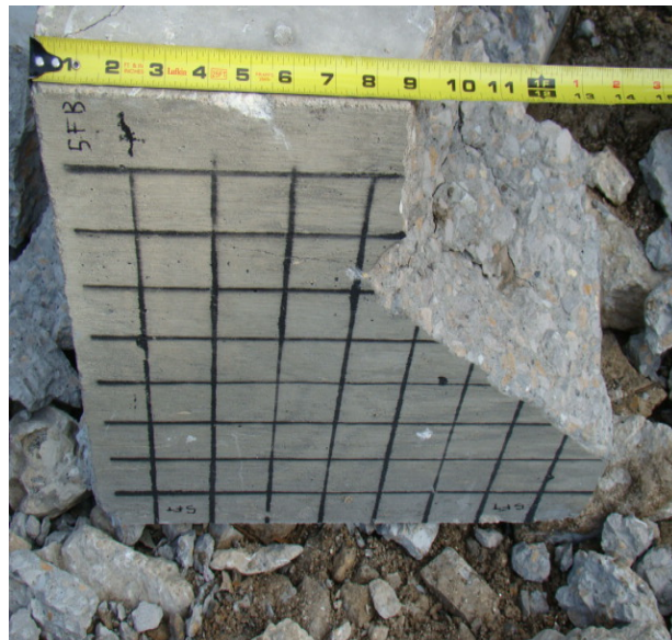
Figure 4.8: Block 5, front face after impact.
