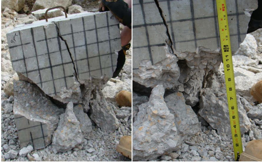
Figure 4.14: Block 9, front face after impact.
