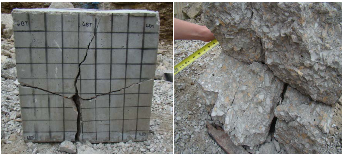
Figure 4.9: Block 6, back face and interior views after impact.
