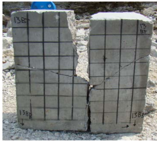
Figure 4.18: Block 13, back face after impact
