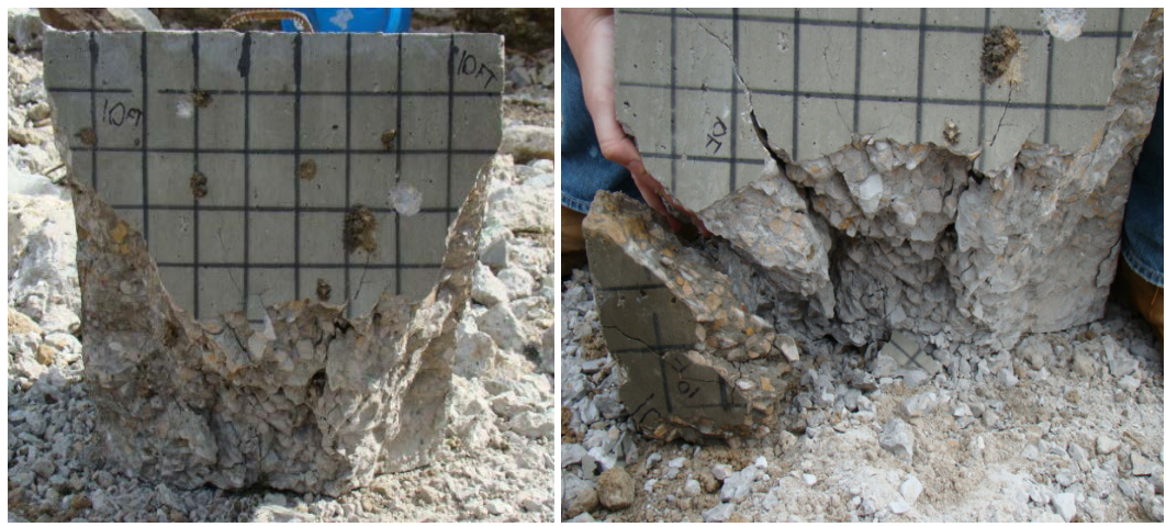
Figure 4.15: Block 10, front face after impact
