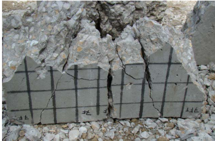
Figure 4.11: Block 7, front face pieces recovered after impact.
