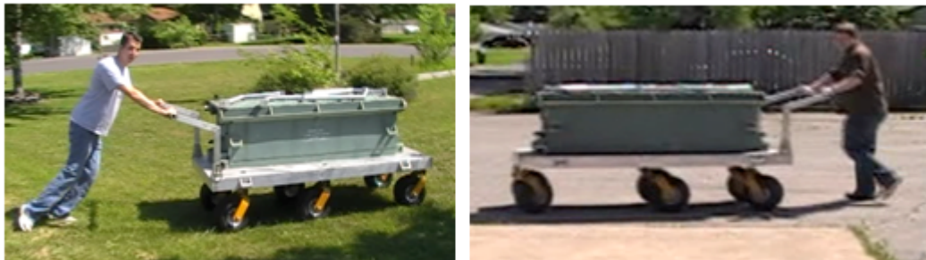
Figure 4.17: Pushing Hand Truck on Grass and Asphalt
