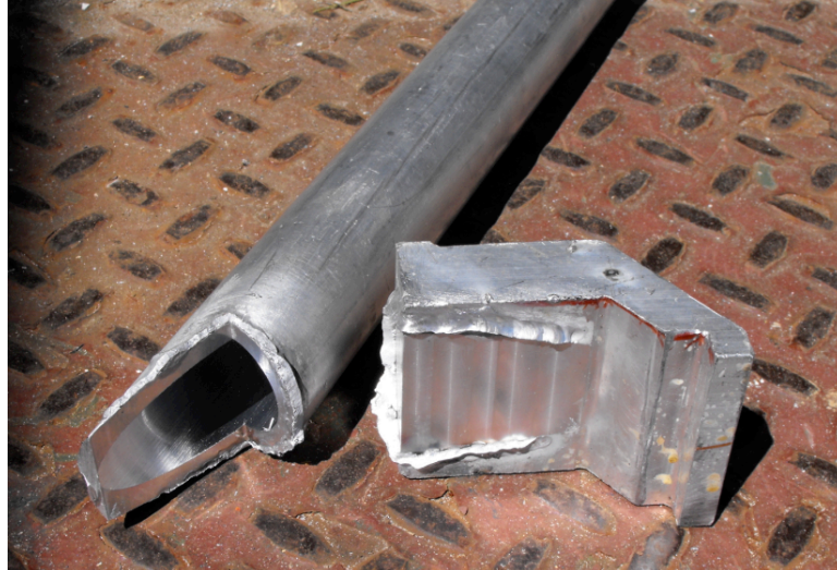
Figure 4.5: Carry Bar Prototype Failure
