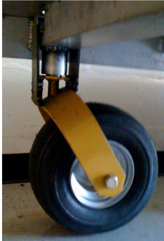
Figure 4.13: Center Wheels of Redesigned Hand Truck
