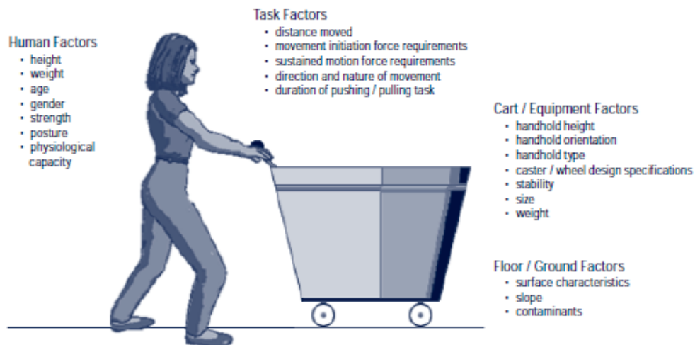
Figure 4.8: Factors Affecting Pushing/Pulling
