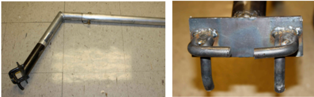
Figure 4.7: Fabricated Prototype of Carry Handle
