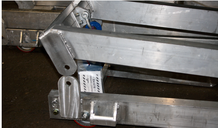
Figure 4.20: Welded Plates for Wire Rope Assembly
