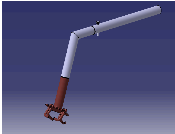
Figure 4.6: Redesigned Carry Handle
