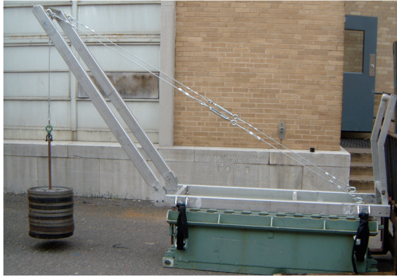
Figure 4.18: First Design of Crane System
