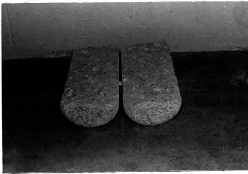
Figure 12. Cylinder Failure Along the Center Line.
