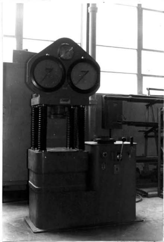
Figure 4. Forney Compression Testing Machine.
