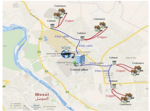
Fig. 3. The proposed FTTN architecture.
