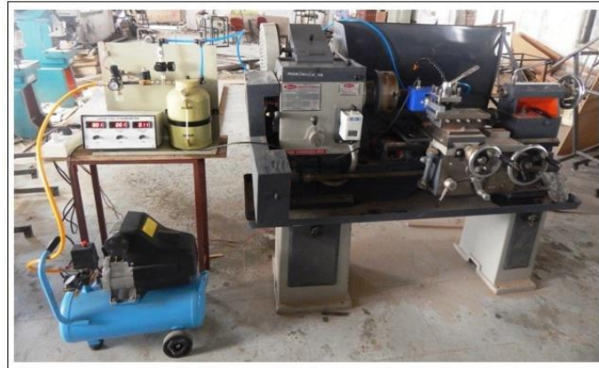
Figure 1. Experiment setup of medium duty lathe machine and MQL system
