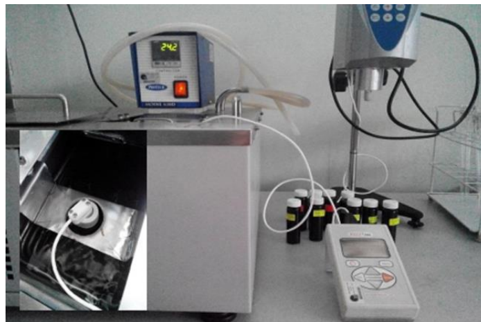
Figure 1. Experimental set-up for thermal conductivity measurement
