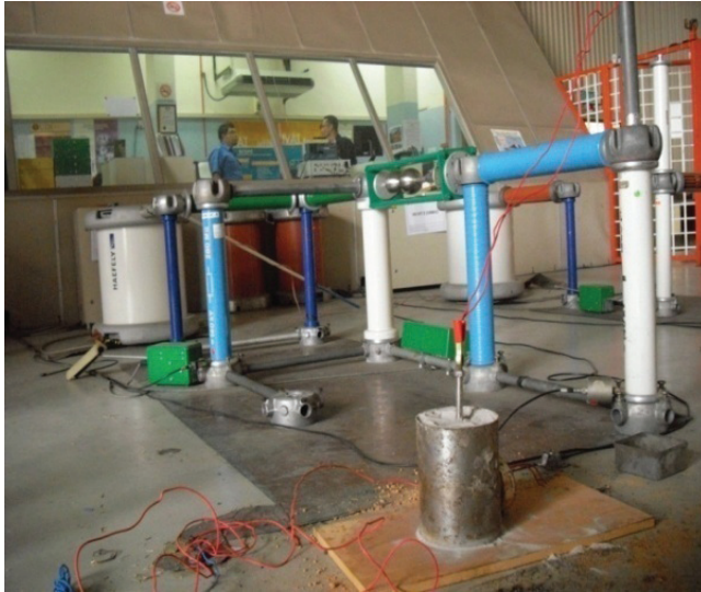
Figure 1. Arrangement for the breakdown voltage under impulse
