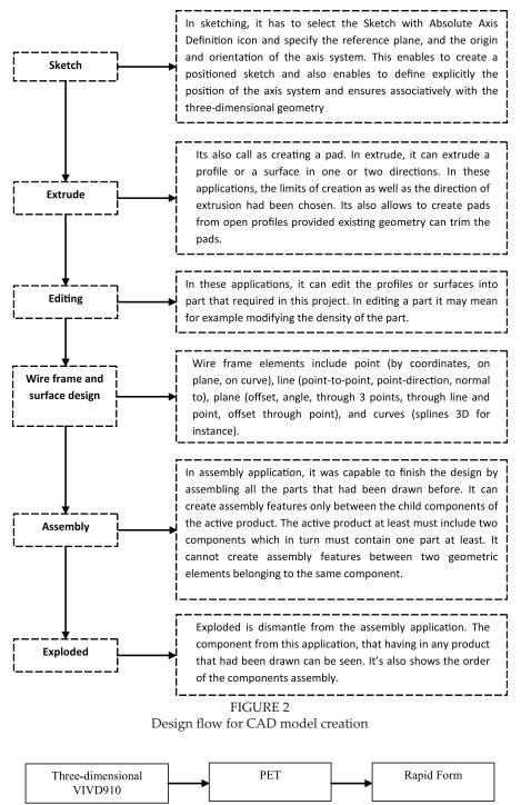
FIGURE 3 Process flow of the reverse engineering method
