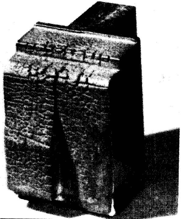
Fig. 4-(b) Severe heat checking in H-21 die after 3000 brass casting cycles
